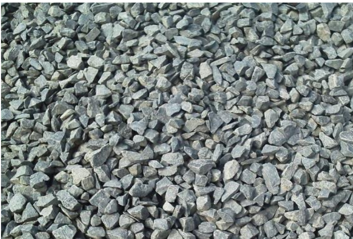
Uniformly sized, highly angular crushed stone
